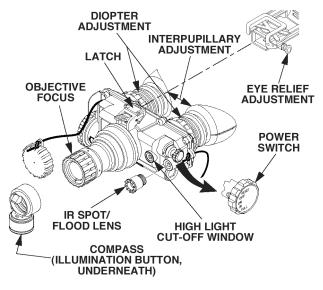
Figure 1-4. Mechanical Controls.
